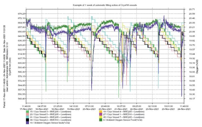
Liquid LN2 level has been compared to the effect on ambient Oxygen levels
