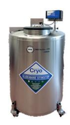
CryoFill on a MVE vessel (Pressure differential measurement)
