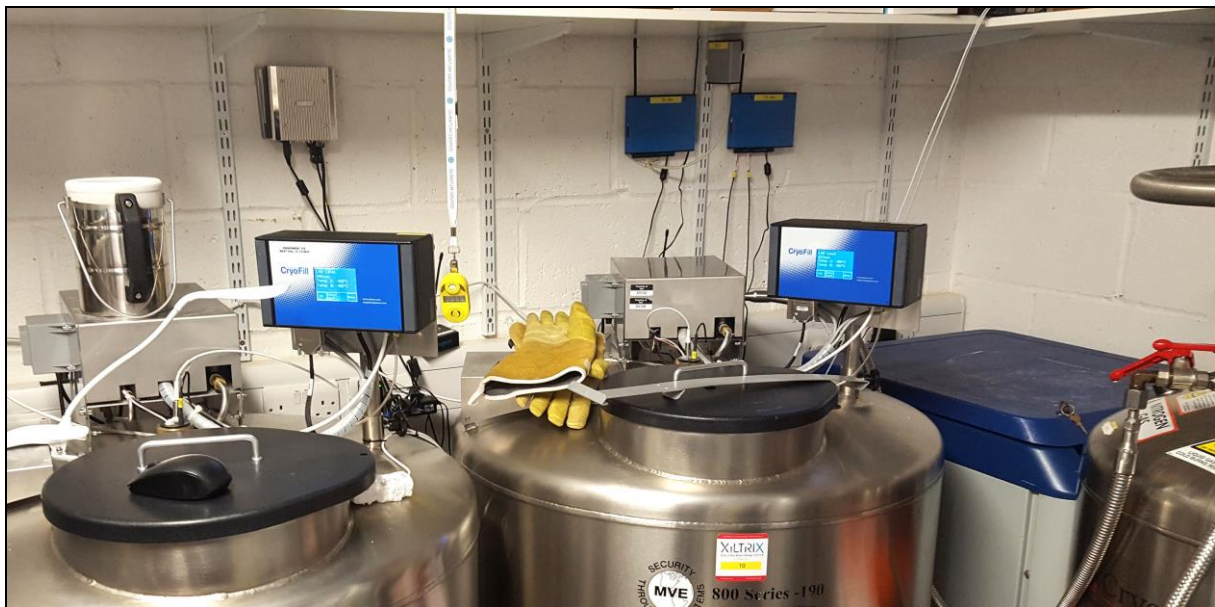
Figure 1: Cryogenic vessels with CryoFill and XiltriX integration
