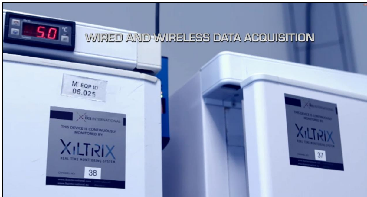
Figure 1: Fridges being monitored in real-time by XiltriX on the Eurofins Microsafe site in Leiden
