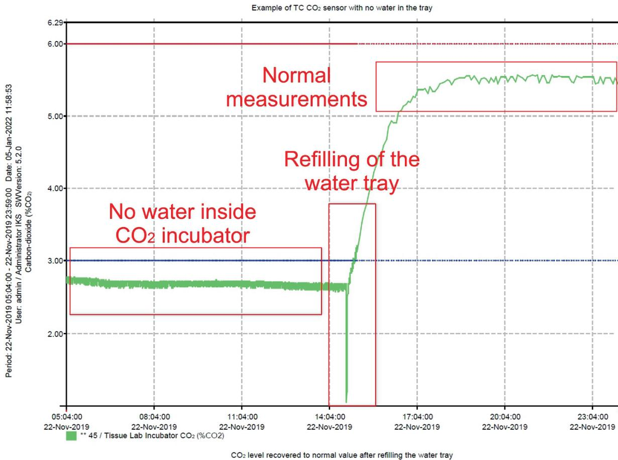
When only monitoring the onboard controller and sensors, in other words the (small) computer that operates the say freezer or incubator, one is led to believe monitoring is in place, but If the controller or circuitry itself fails, no alarm will be sounded. There is no independent referee in place nor in control.
