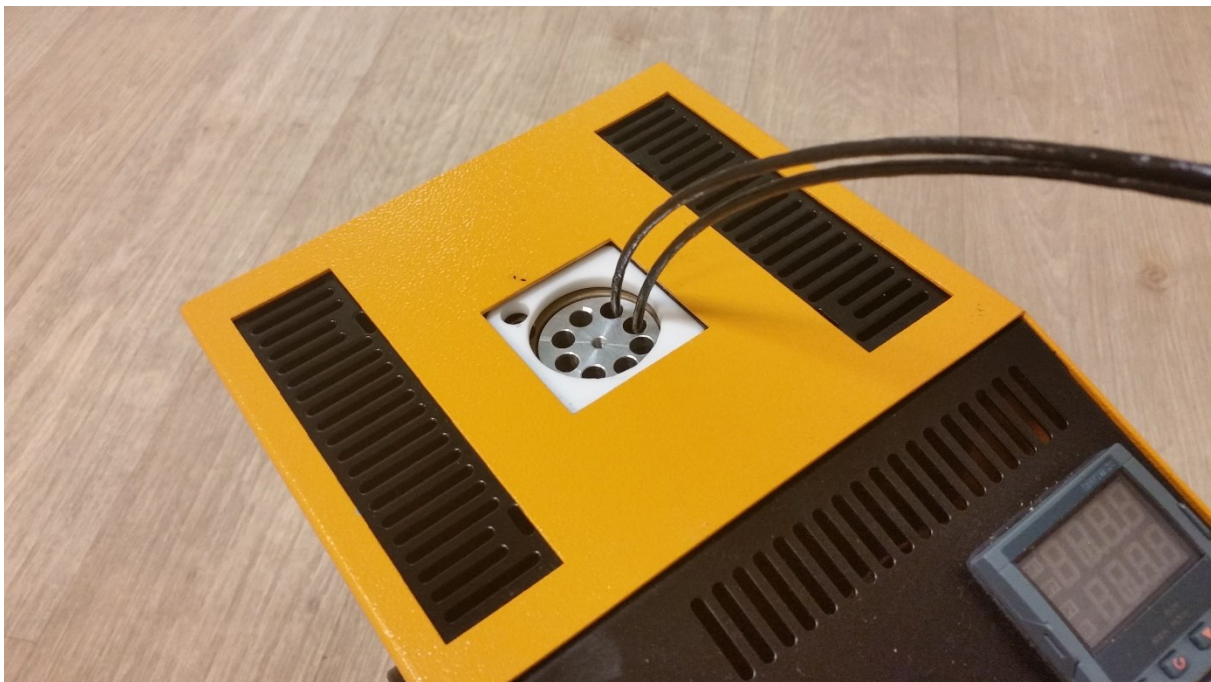
Figure 1: Placing sensors in a block oven is a good example of creating a stable environment to calibrate sensors in
