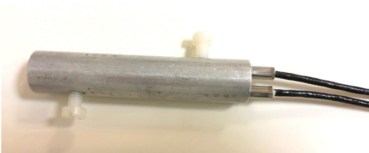
Figure 2: When sensors cannot be easily removed placing an aluminium block inside a device will greatly improve stability of the measurements, resulting in a lower uncertainty
