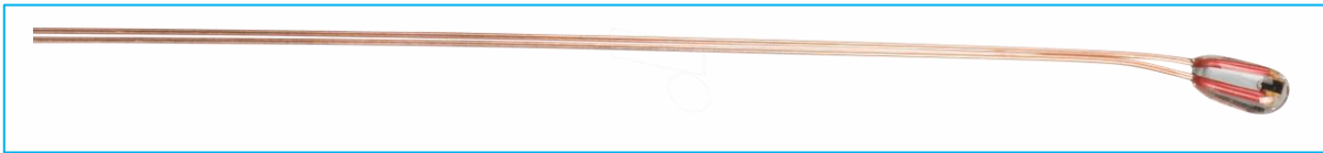
Figure 2: Example of a very small NTC sensor used for measuring temperature inside droplets.
